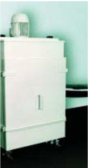
After a knife box exchange, the used knives are usually extremely dirty. PUTSCH® Automatic Cleaning and Sorting Machines RSA remove scaling, corrosion and beet-residue from the surfaces of the Koenigsfelder knives. This cleaning operation improves the cassette quality and protects the Automatic Knife Reconditioning Machines against excessive wear.
