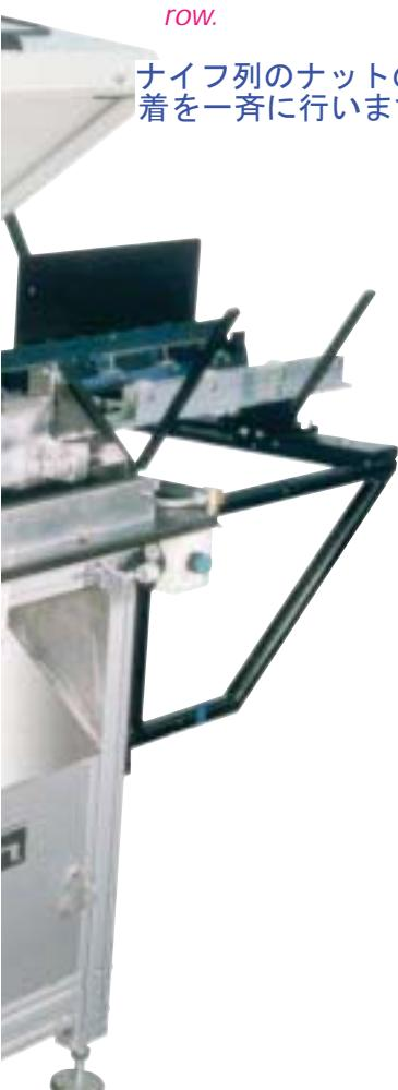
The PUTSCH® automatic wrench simplifies and speeds up the exchange of knives in the knife boxes from PUTSCH® drum slicers TSM 2200-22-600 and TSM 1800-18-600. Depending on type of drum slicer up to 198 knives need to be exchanged and 396 nuts to be loosened and fastened per complete set of knife boxes. The loosening and tightening of the nuts is done in a fast, uniform and precise manner.
